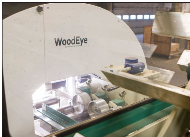
The WoodEye's automated scan system provides us a more consistent product.
