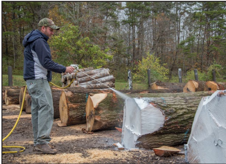
Adam Ward spraying wax on the ends of veneer logs, prior to an export shipment.
